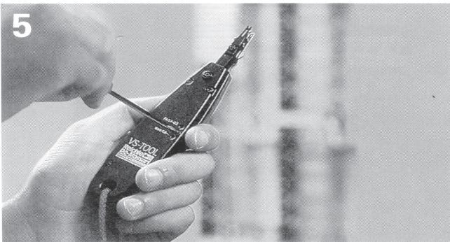
■ Select the diameter of the conductor to be wired.
