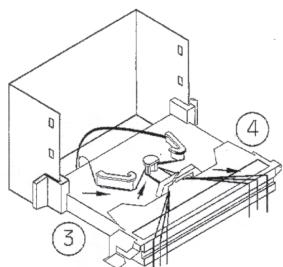
3. Put the wires in accordance with the arrows through special wire deflectors, as indicated in figure
