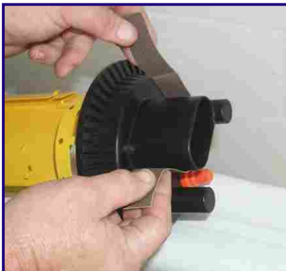
4 Abrade the selected open port. (Not required when using a rubber cablegrip)
