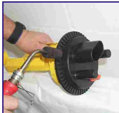
5 Flame brush port prior to applying heatshrinkable sleeve. (Not required when using a rubber cablegrip)
