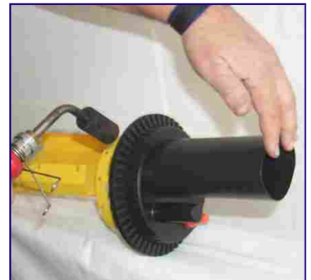
6 Place heatshrink over the open port and shrink down onto port, leaving approx 10mm unrecovered at the end of the port. (Not required when using a rubber cablegrip)
