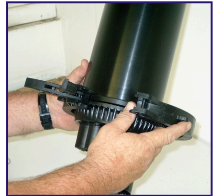
6 Open the swing clamp and remove the cover.
