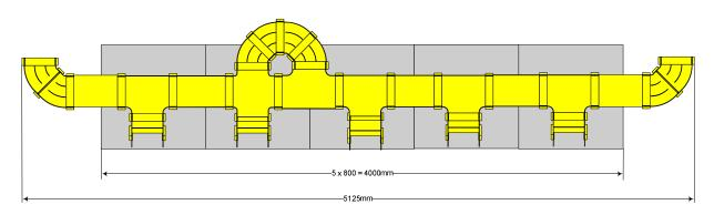
Important: The sample (pictures) is build-up with Raceway 100x100mm elements. If you work with other dimensions it could be different, between the two cross is a small piece of duct and a second joint is needed.
